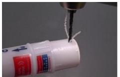
Using a (4.5mm) drill bit, carefully drill out the two retaining clips as shown. There are no internal components beneath these clips.
