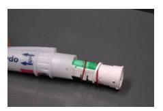
Remove the PCB & Battery assembly from the cap and then disconnect the battery from the PCB by removing the connector as shown below.
