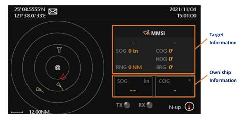
Radar View displays own ship and target ships' statuses, and their correlations. It is a proportional chart scale showing the current ratio displayed. The distance between the inner and outer circles (1 grid) is the number displayed on the scale at left bottom. You can adjust the scale to display ships in different distances.
