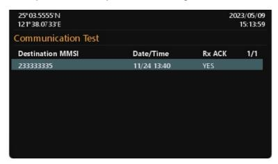
Press to start the communication test. The system will show Target List that only has targets with Class A type. Use direction keys to select a target and then press
