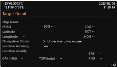
Use direction keys to continue reading the dynamic and static information of the selected vessel.
